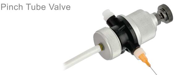
Engineered for precise control of semi-viscous liquids including mixed two-part component fluids and cyanoacrylate. The only part of the valve making contact with the fluid being dispensed is the disposable pinch tube assembly.
