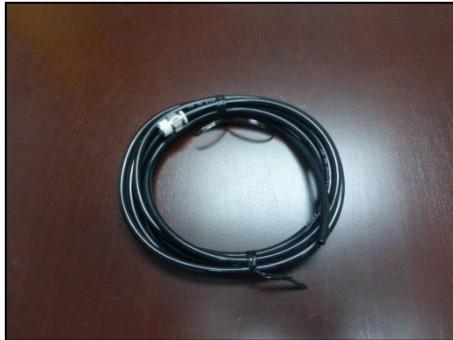
Controller-to-Compressor Air Line
