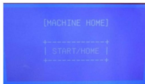
Teach Pendant display will show START/HOME, you have finished the alignment.
