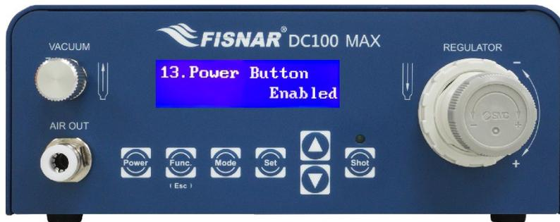
1. When the Power Button page is displayed, press the
