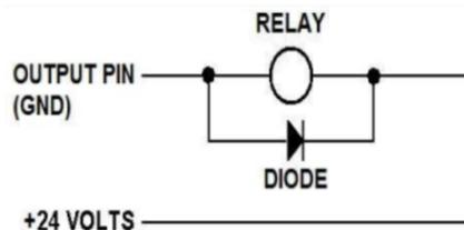
Installation of Diode
