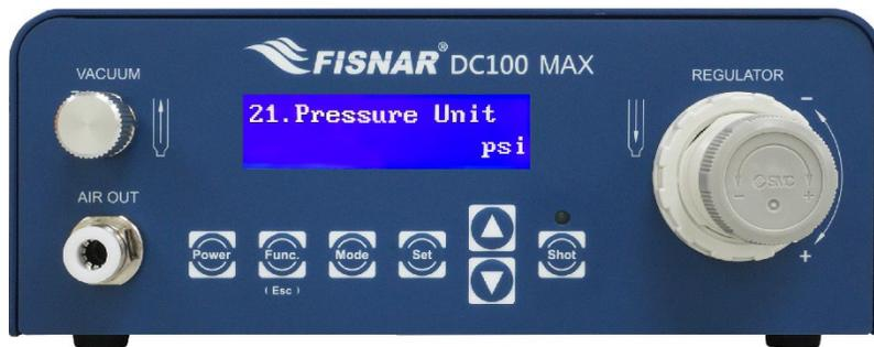
1. When the Pressure Unit page is displayed, press the
