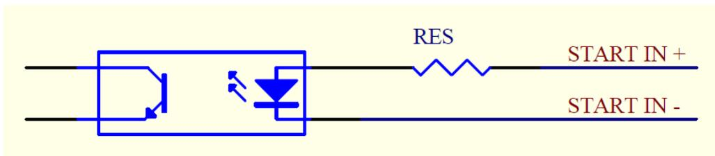
Example of I/O input port driving (pin #8)
