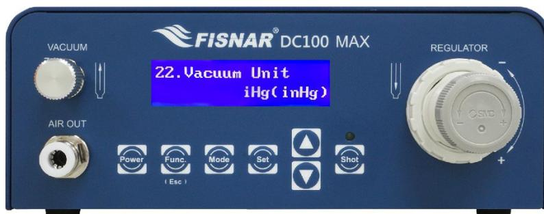
1. When the Vacuum Unit page is displayed, press the
